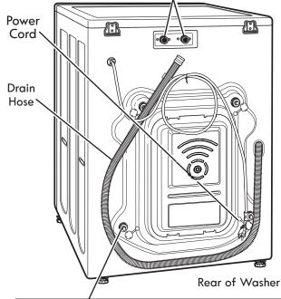
Shipping Bolts/Retainers (4) NOTE: Bolts/Retainers MUST be removed prior to operation. Keep for future use.
